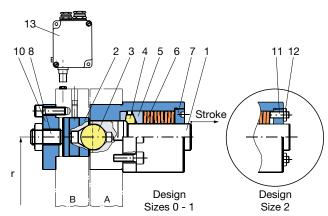
Fig. 1: EAS®-element engaged
