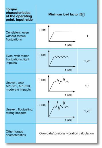
We recommend carrying out a torsional vibration calculation (TVC) for coupling dimensioning on drives with internal combustion engines.
